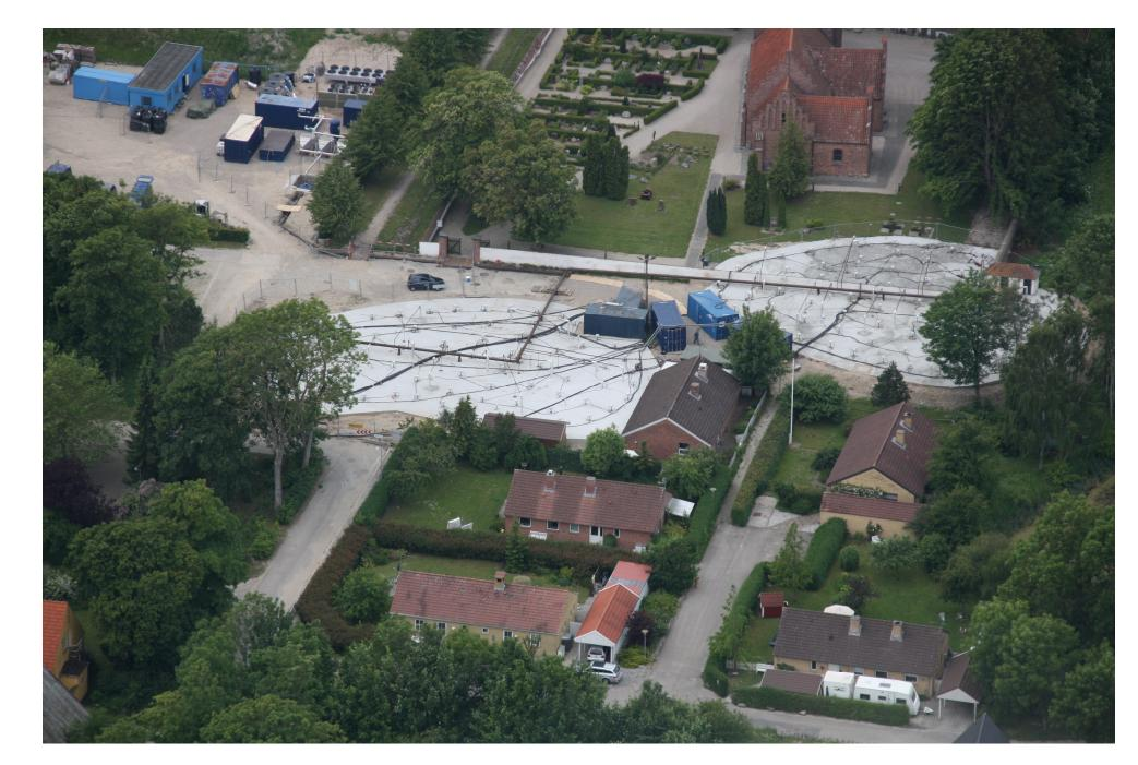
by the thermal conductivity of the soil. Increasing temperatures drives the pollution towards gaseous form and produced steam and polluted gas is extracted through ventilation wells.
