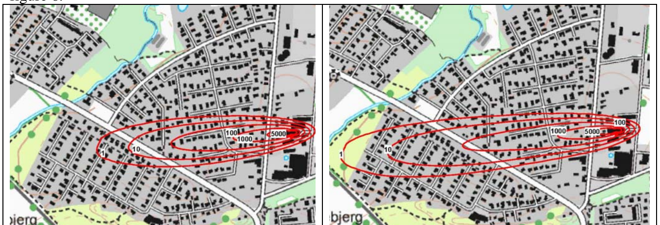
Figure 6. Contamination distribution 50 years after excavation of the contaminated soil from the main source area including remediation of the groundwater aquifer.
