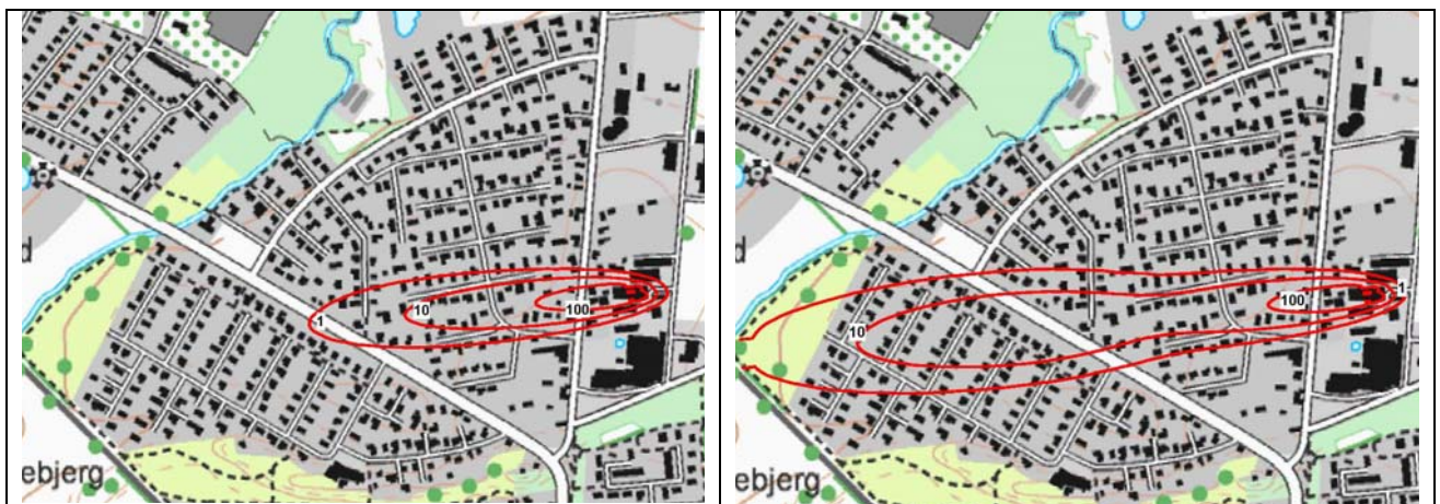
Figure 5. Contamination distribution 50 years after 94% remediation in the source area.
