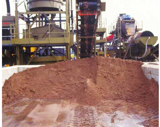
Left: debris on a former gasworks site; right: output from a soil washing plant. Credit: Steve Wallace; use Courtesy of National Grid Property
